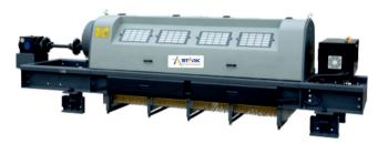
This new generation of high-quality electronic jacquard machine is designed specially for high-speed looms. based on years of mature technology, the exterior and control system is upgraded and driving system is optimized and improved, Embedded intelligent control module and touch-screen human-computer interaction interface has better experience. Transmission friction is small and stable. It can meet the requirement of running in high-speed and long-term.
